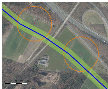
Figuur 5 Scenario 2: Mastbreuk, effect gondel
