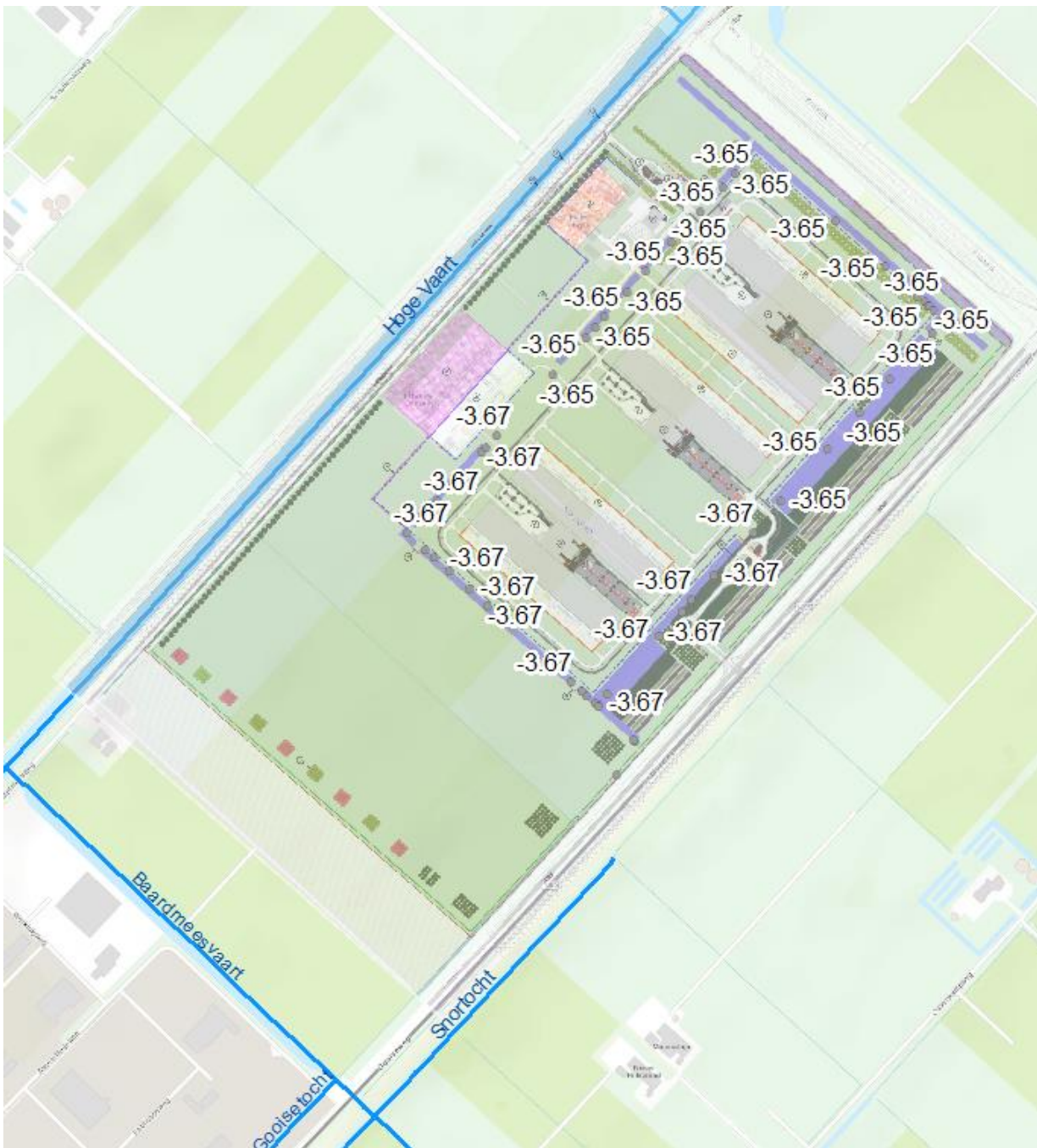
Figure 12. Peak water levels modelled in the design situation for a T=100 urban precipitation event on the datacenter project site.
